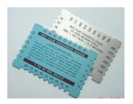
To help insure proper coverage an inexpensive wet film gauge can be purchased and used. The approximate wet adhesive thickness should be 10-14mils.
