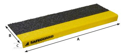
Safeguard® Hi-Traction® Step Covers are not load-bearing but are installed over existing steps. They are sized to meet your specifications with Length (A) and Depth (B) made to order. A standard 1" (25 mm) vertical lip (C) wraps over the leading edge where most slips occur.
