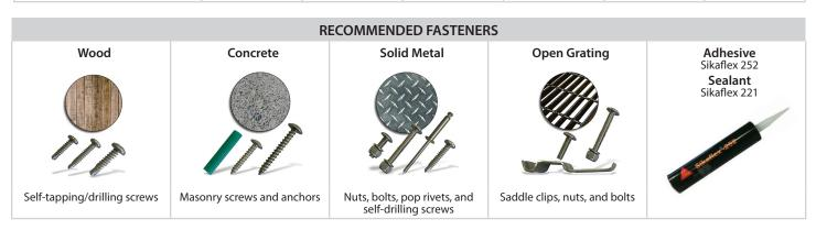
Select the appropriate fastener for the substrate to be covered. A combination of mechanical fasteners and adhesive may be used. Sikaflex 221 sealant may be used to seal edges to deter corrosion. Fasteners and pre-drilled/slotted holes are available upon request.
