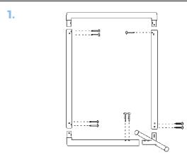
Connect tubular frame parts as shown using screws provided. Only one leg is required if directional flexibility is desired. With one leg you can easily flip your Panel from vertical to horizontal.
