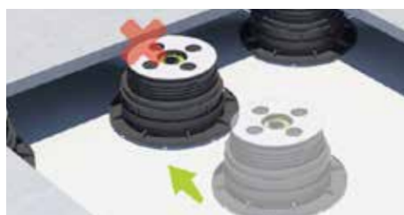
2. Place the pedestal at the level of the adjacent tiles in order to correctly modify the height.
