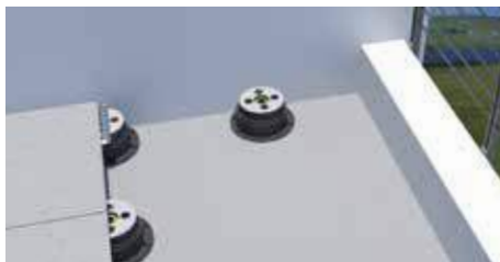
2. Place the pedestal with the cut side against the wall.
