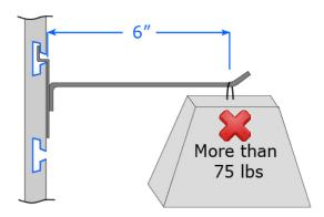
If the load increases to more than 75 lbs, the slatwall could break
