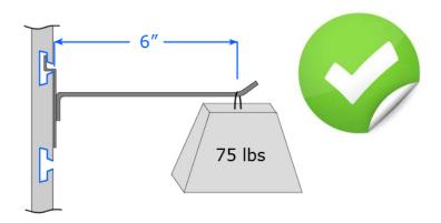
SlatWall MX<sup>™</sup> Strip can hold a 75 lbs point load hanging at a 6" distance from the slatwall face:
