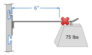
If the 75 lbs load moves further away than 6" from the slatwall face, the slatwall could break
