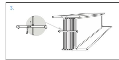
Screw wheel base to bottom of panels into square nuts. Image shows approximate placement. The bottom of panels are pre-drilled. Slide square nut to this location. Attach wheel assembly with large screw using allen wrench. Keep pressure on wheel bar will help to maintain perpendicular placement.
