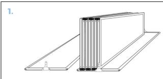
Gently place both end panels on the ground and lift partition bundle (placing it on it's side) on top of one of the end panels.\*
