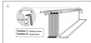
Line up bracket on end panel to the holes on the outside piece of panel bundle. Screw two bolts into each bracket on the end of the panels as shown.
