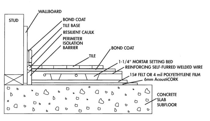
Tile Floors over 1-1/4" Mortar Setting Bed on a Concrete Slab
