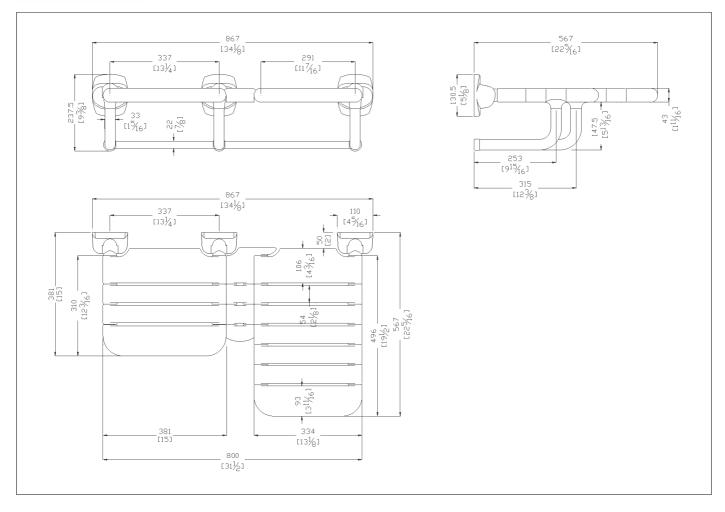
Double folding seat with nylon slats made of zinc-plated steel pipe, coated with antimicrobial, biocompatible, warm to the touch vinyl
