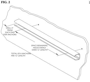
2. Drill holes in centerline of retainer using 1/4" drill bit. Position retainer on wall allowing for end caps/corners. Level and mark holes. See Figure 2.
