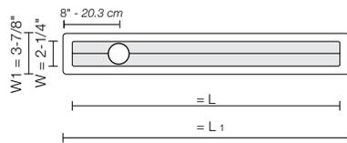
**8.7 Schluter®-KERDI-LINE** Bonding flange - stainless steel - off-center outlet
