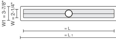
**8.7 Schluter®-KERDI-LINE** Bonding flange - stainless steel - center outlet
