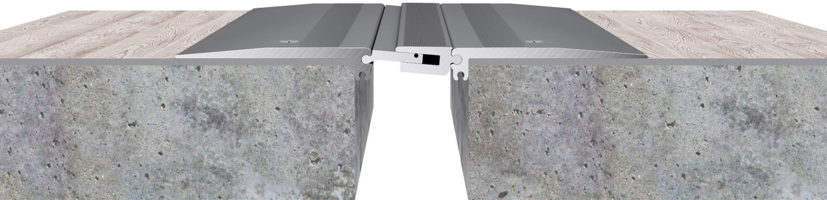
This all-metal, surface-mounted cover is resistant to rolling loads, distortion, and wear. It includes slip-resistant serrations and is intended for interior or exterior applications where minimal movement is expected. The unique interlocking cover design allows for horizontal movement in the floor slab, as well as some vertical deflection and is extremely low maintenance.
