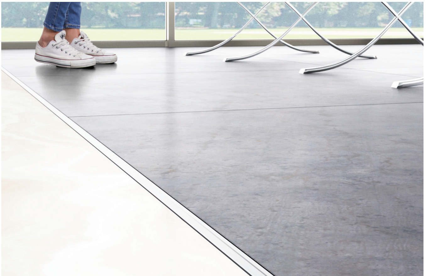
DILEX-EDP stainless steel movement joint profile used to separate individual fields in the tile covering, and accommodate horizontal movement.
