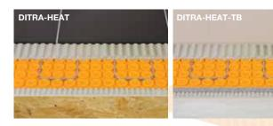
**Schluter®-DITRA-HEAT** and **Schluter®-DITRA-HEAT-TB** are polypropylene membranes with a cut-back stud structure and an anchoring fleece laminated to the underside. Both systems are designed to secure the DITRA-HEAT-E-HK electric floor heating cables in place, and provide uncoupling, waterproofing, vapor management and support to ensure a long lasting installation. The DITRA-HEAT-TB also features a thermal break that provides up to 70% faster warm-up times over concrete substrates.
