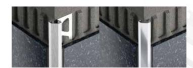
**Schluter®-DIADEC** is a finishing and edge-protection profile for tiled edges and outside corners of tiled surfaces. The reveal of the profile forms a 45° beveled edge. DIADEC features integrated joint spacers that establish defined joint cavities between the tile and the profile.
