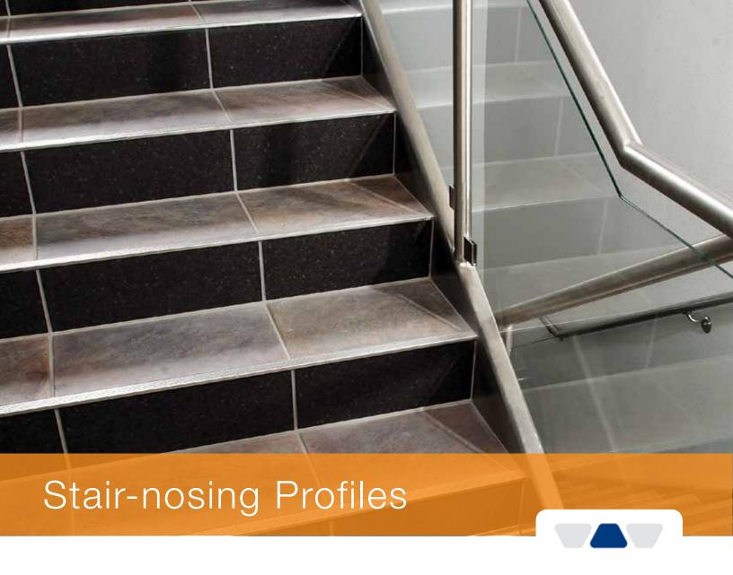
Tiled stairs edges that do not utilize appropriate trim pieces are vulnerable to chipping and breaking and create a slip hazard, especially in exterior applications. Schluter® stair-nosing profiles protect exposed tile edges and improve safety on tiled stairways by providing slip-resistant wear surfaces and increased visibility in both residential and commercial applications.
