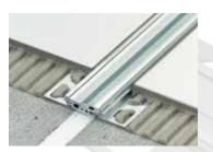
Schluter®-DILEX-BT is an expansion joint profile made of anodized aluminum that bridges expansion joints and accommodates horizontal movement. DILEX-BT protects tile edges and is suitable for tile surfaces exposed to foot traffic as well as vehicular traffic and is, therefore, suited for use in warehouses, production facilities, shopping centers, airports, train stations, and parking garages, or for coverings cleaned with machines.
