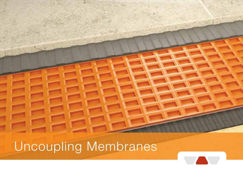
Today's construction methods, which include the use of lightweight materials, have made the installation of hard surface coverings particularly challenging. Because of the differences in material properties the substrate and the tile layer expand and contract at different rates, creating stresses in the assembly that can ultimately result in damage to the finished tile surface.
