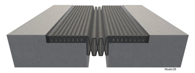
This parking cover has an EPDM seal that allows for movement, while the integral nosing eliminates the need for elastomeric concrete. During installation, the cover is bonded into a high-strength epoxy bedding and is sealed on each side with a urethane sealant, resulting in a durable and watertight system.
