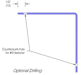
Standard spacing: 1" (25) from each end and spaced evenly not to exceed 36" (914) oc
