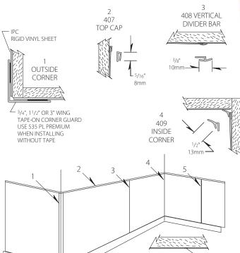
FOR .080" THICK SHEET, USE 417 TOP CAP, 418 VERTICAL DIVIDER BAR AND 419 INSIDE CORNER
