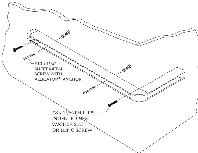
3. Drill marked holes on wall using a 1/4" drill bit and position Alligator anchors into holes. Mount retainer on wall and tighten screws to secure. Slide end caps and corners onto the retainer and secure, leaving a 1/16" gap between end caps/corners and retainer to allow for adjustment. See Figure 3.
